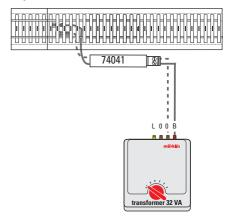
FCC Feeder Wire Set: This feeder wire set is to be used only to make connections to your Märklin H0 model railroad!
