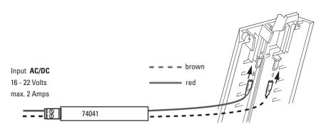
Connections on the underside of the track
